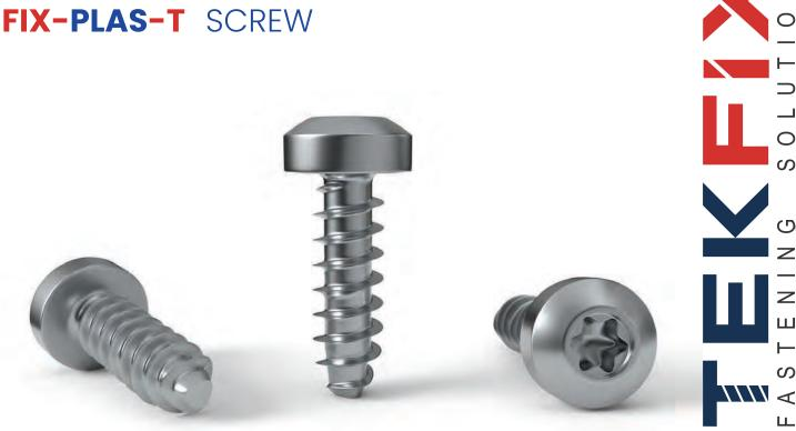
FIX - PLAS-T screw is designed to facilitate thread-forming in less-compressible plastics while providing high resistance to strip-out and pull-out. The single-lead design and narrow helix angle lowers drive torque and failure torque in stiffer plastics.
